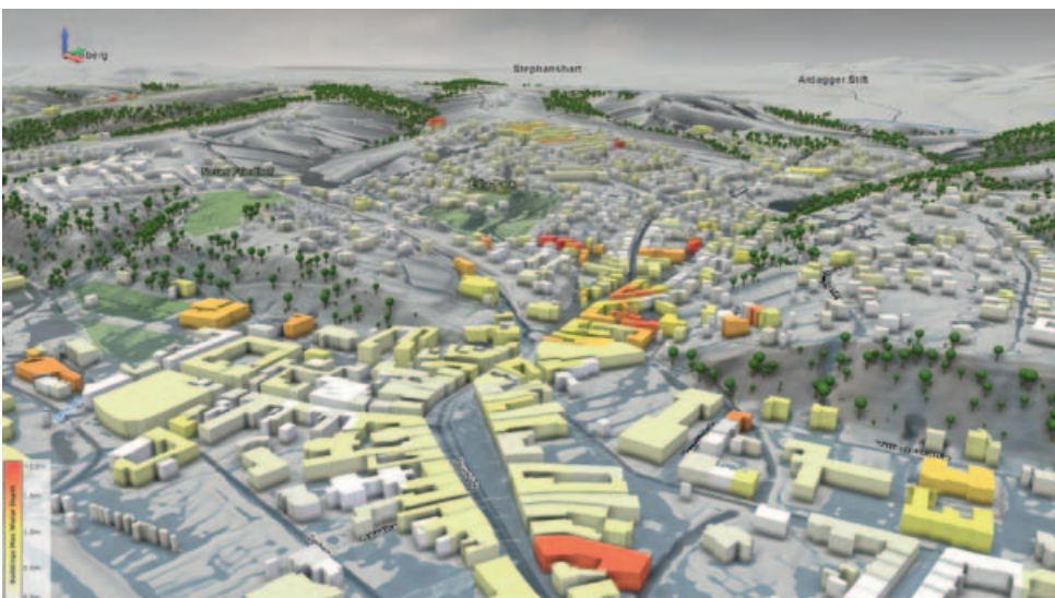
▲ Figure 1: Buildings are colour-coded according to the estimated flood damage in a heavy rainfall scenario.
